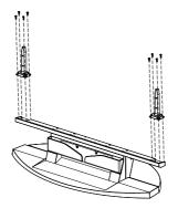
2 Using the 4 screws for securing the Stand Pegs and the Monitor, firmly attach the Monitor to the Stand Pegs. (The exterior of the SET may be different than the picture.)
